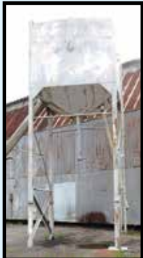
SANDBLAST GRIT TOWER
