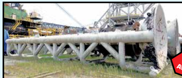
CONMACO 6850 OFFSHORE PILE HAMMER
