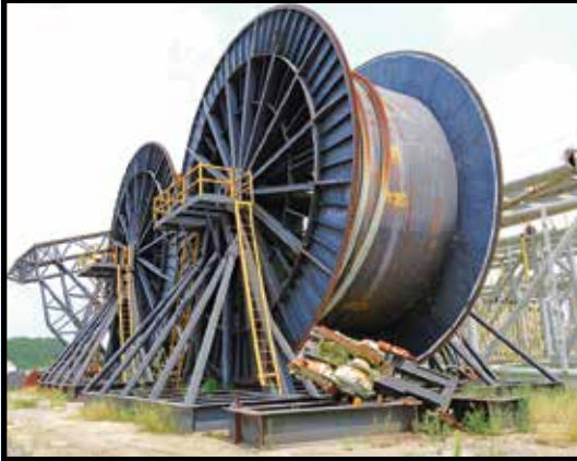
OFFSHORE PIPE LAY REELS
