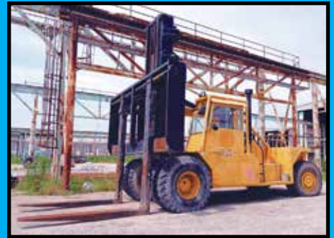
90,000 LB. CAP. TAYLOR DIESEL FORKLIFT
