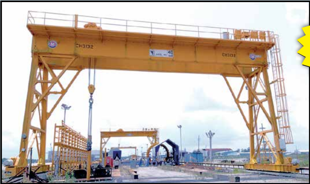
LANDEL 40 T. TRAVELING GANTRY BRIDGE CRANE
