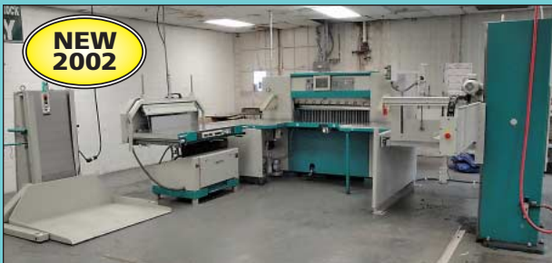
Overall View 52" Perfecta Model 132 IVC Paper Cutter w/ Jogger, Lift and Unloader
