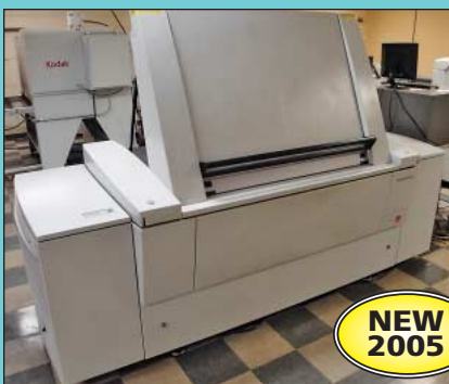
Kodak Model 3244AL Trendsetter News Platemaker w/ Autoloader Plate Feature
