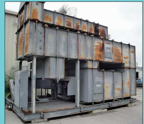
Grace / Tec System Phoenix High Efficiency Thermal Systems Gas Fired Fume Incinerator
