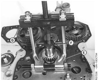
E-D01218AA Pulling attachment F-Disc G-D01200AA Push Puller
