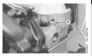
cooling system, loosen coolant temperature sensor or plug at the rear of cylinder head (B) to allow air to escape.
