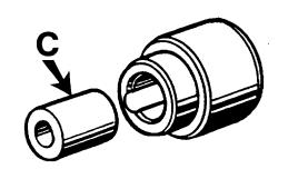
NOTE: KJD10164 tool set contains also a spacer (C) to be used only on old applications with short nose crankshaft (35 mm length).
