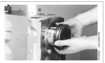
6. Remove connecting rod and piston assembly through the cylinder liner.
