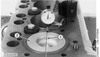
1—Centerline of cylinder liner bore 2—Piston at "TDC"
