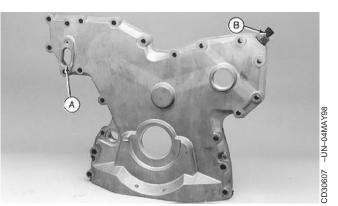
Timing gear cover with auxiliary drive
