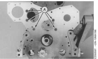
A—Countersunk screw B—Oil by-pass valve C—Stud location D—AT21191 Plug (5/16") - Qty: 6 E—AT22919 Plug (3/8") - Qty: 2 F—T23442 stud - Qty: 3 G—R79854 Bushing
