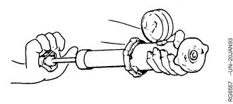
Pressure Testing Radiator Cap
