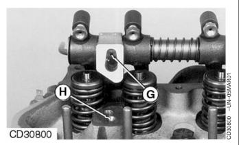
G—Oil supply hole in rocker H—Oil supply hole in cylinder arm shaft head
