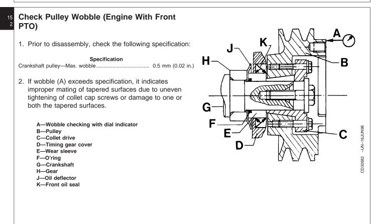
**Remove PTO Pulley**
