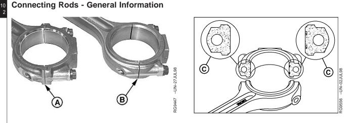
A—Tongue-and-Groove Rod (early engines) B—PRECISION JOINT Rod (later engines) C—PRECISION JOINT detail
