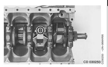
IMPORTANT: Before tightening rear cap screws, ensure that rear thrust washer of cap is aligned with rear thrust washer of block.
