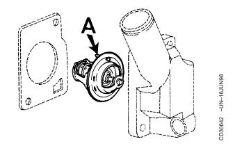
Deaeration is normally accomplished by the jiggle pin (A) in thermostat flange area. However a pocket of air can stay on the top rear of engine. When refilling
