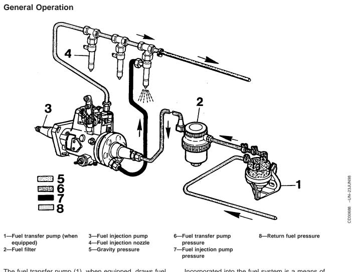
The fuel transfer pump (1), when equipped, draws fuel from the tank and pressurizes it. This pressure permits the fuel to flow through the filter (2) and charge the transfer pump of the injection pump (3).
