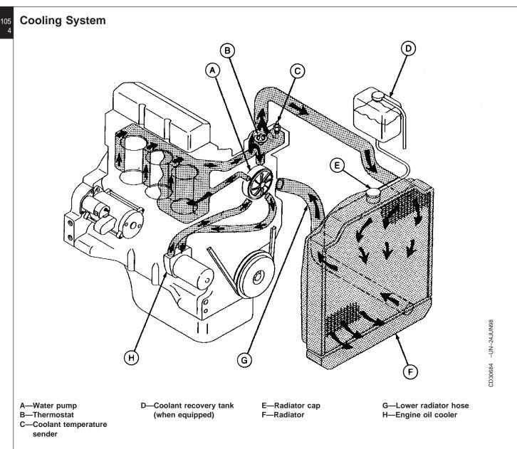
The principal components of the pressure cooling system are the radiator, water pump, multi-blade fan and thermostats.
