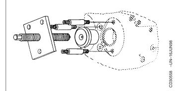
Install camshaft bushing using JDG739B as follows:
