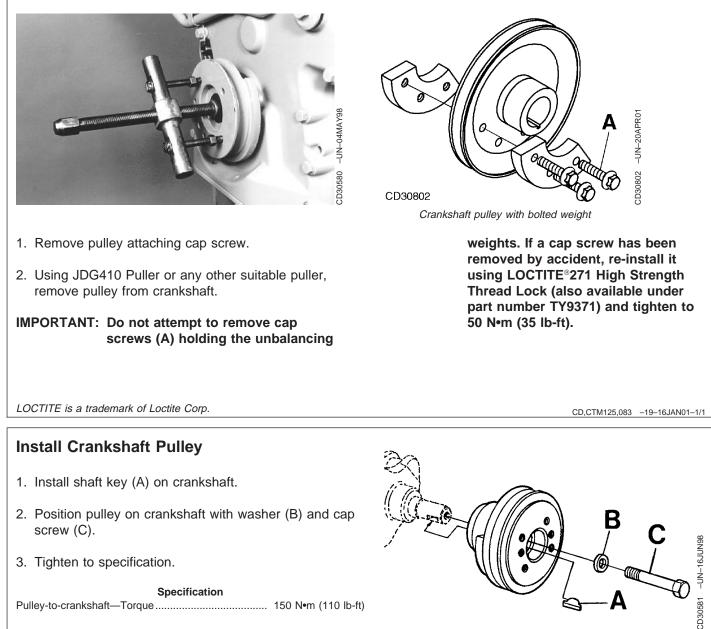
**Remove Crankshaft Pulley**
