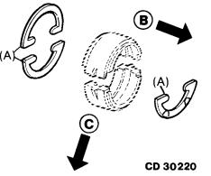
A—Oversized thrust washers **B**—Front of engine C-Rear bearing cap side
