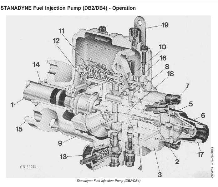
1—Drive shaft 2—Distributor rotor 3—Hydraulic head 4—Delivery valve 5—Transfer pump
