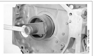
3. Slide driver onto guide and gradually tighten the cap screw or nut until driver bottoms.
