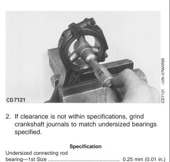
NOTE: Undersized crankshafts may be also available through the regular service parts channel.
