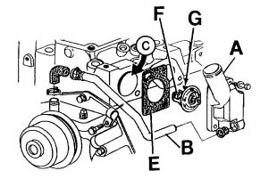
A-Thermostat cover B-By-pass tube
