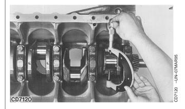
NOTE: Before measuring, connecting rod cap screws must be tightened according to specifications.
