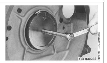
2. Secure the assembly with a clamp then gradually tighten the screw until wear sleeve is extracted.
