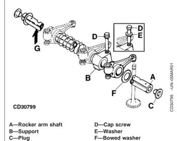
NOTE: Effective with following engine serial numbers, shaft (A) and cap screw (D) with washer (E) have been replaced by a new shaft and flanged head cap screws.
