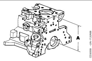
A—Distance between crankshaft bore center line and block top face
