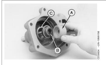
Support water pump on shaft end. Using the installation tool (A) included in the seal kit, install water pump seal (B) over shaft until seal bottoms on shoulder (C) of housing. -UN-T9MAY98
