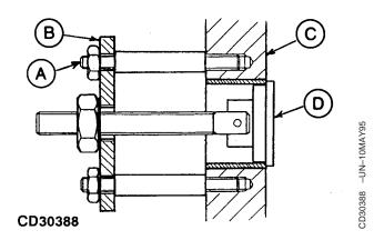
Extract camshaft bushing using JDG739B tool as follows:
