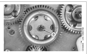
7. Install washer, with sharp edge toward timing cover, and bolt (B) then tighten to specification.
