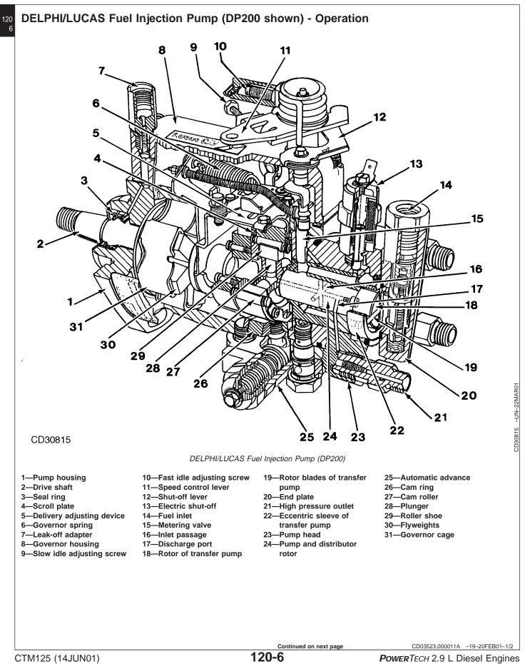
061401 PN=232 IMPORTANT: Remember that all adjustments to the injection pump - except for slow idle - must be carried out on a test bench by a specialist injection pump repair station only. Internal adjustments in the field are not permitted, as this pump is a sealed unit.
