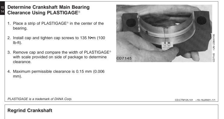
If journals are worn, tapered, out-of-round, scored or damaged, the crankshaft journals can be reground and correct undersize bearing inserts installed.
