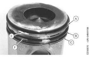
A—Top ring B—Second ring C—Oil control ring D—KJD10140 Piston Ring Expander E—Blue mark F—Yellow mark
