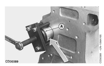
IMPORTANT: Bushing must be installed so oil supply hole (arrow) aligns with oil drilling in block bore.
