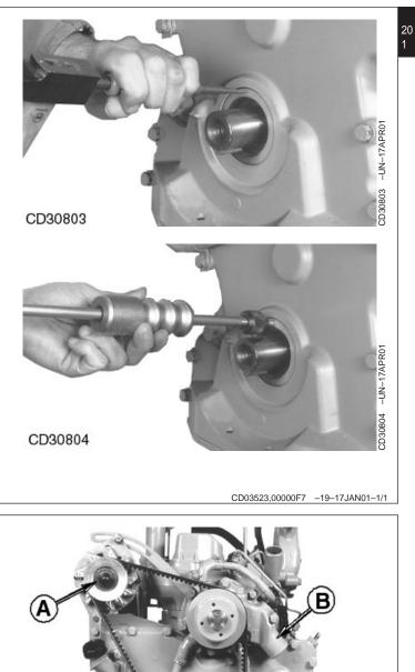
Remove Timing Gear Cover
