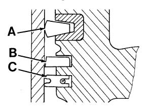
Use KJD10140 or any other suitable piston ring expander for a proper installation and to prevent any damage to the piston.
