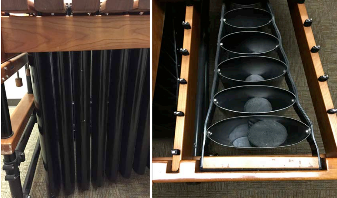
Figure 2.4: Side and Upper view of oval resonators (Pictured, Marimba One 3000 series).
