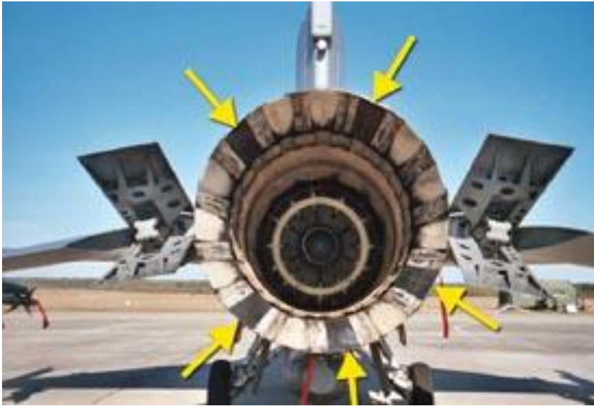
An F-16 Fighting Falcon F100 engine exhaust nozzle with five A500 ceramic matrix composite divergent seals, identified by the yellow arrows. (Air Force photo)
