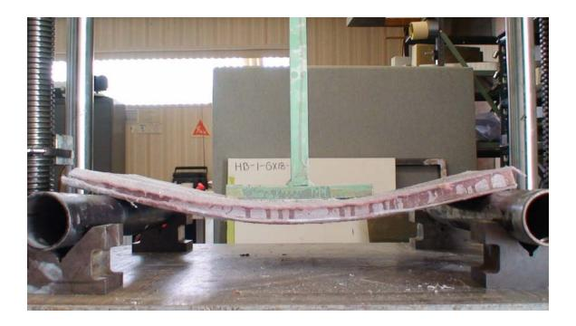
Figure 3. Structural Testing of Steel/Composite Interface Joint
