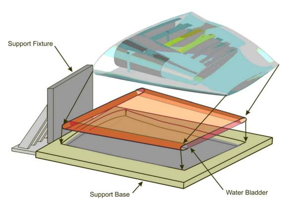
Figure 4. Plan for Full-Scale Static Testing
