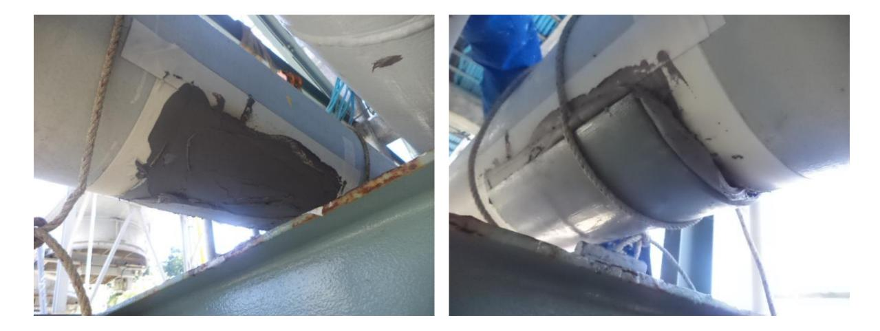
BELZONA® Repair • Protect • Improve Bond metal plate with corroded pipe
