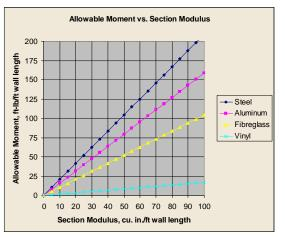
The chart to the left<sup>1</sup> shows the relationship between the section modulus and the allowable bending moment for a selection of sheet pile manufactured in (4) different materials, using the formula above. It can be seen first that, for a section with the same section modulus, sections manufactured from pultruded fiberglass have a higher allowable bending moment (by a factor of more than six) than comparable vinyl sections.
