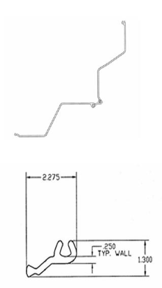
Composite Z corners are generally installed with the last "Z" sheet to be driven. e.g. The corner is hand threaded into the "Z" shape prior to setting the last "Z" shape in a wall
