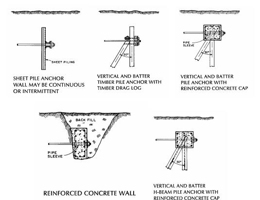
(5) TYPICAL SHEET PILING BULKHEAD ANCHORING METHODS UTILIZING A CONVENTIONAL GALVANIZED TIE-ROD.
