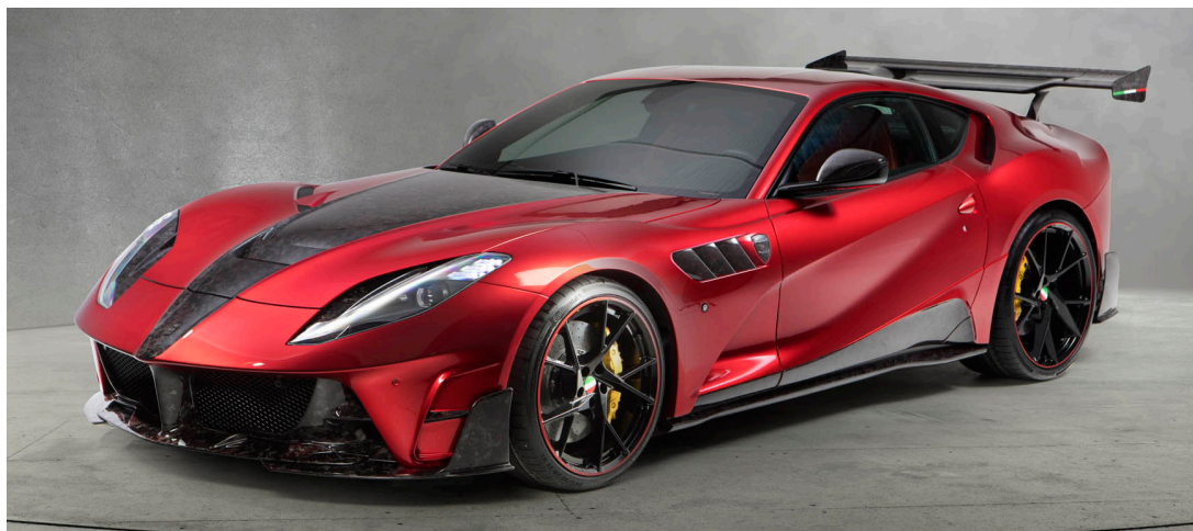
Photo of the Mansory Stallone 812: the car body is entirely made in Polynt-SMCarbon®. Photo by Mansory
