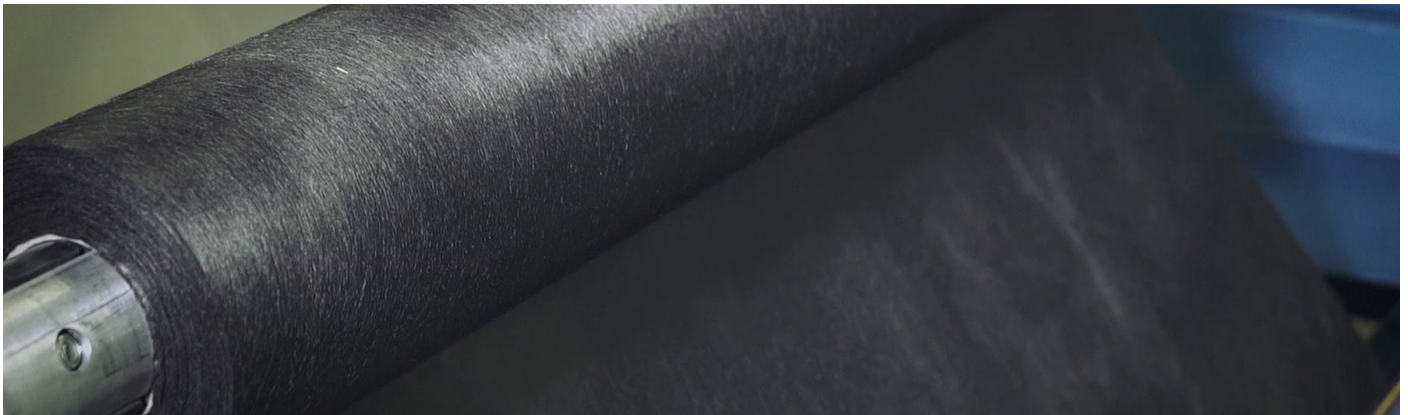
Detail of recycled carbon fiber veil for surface improvement (20 gr/m)
