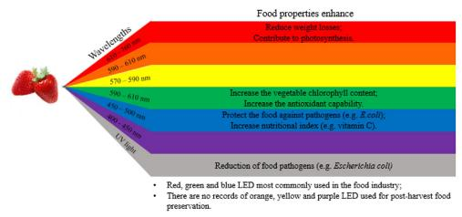
Fig 1. LED and UV-LED wavelengths and applications over food properties.
