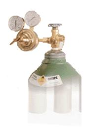
If there is any question as to the suitability of a regulator for a particular gas, check with your vendor for advice. After the regulator is attached, the cylinder valve should be opened just enough to indicate pressure on the regulator gauge (no more than one full turn) and all the connections checked with a soap solution for leaks. *Never* use oil or grease on the regulator of a cylinder valve.
