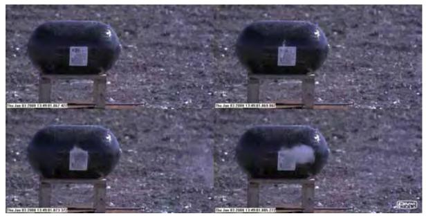
Figure 8. High-Speed Video Frames of 10,000-psig Type 4 Cylinder Penetration Test.
