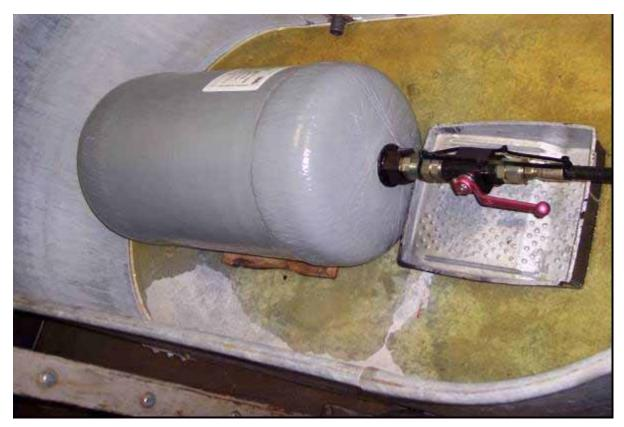
Figure C-6. 5,000-psig Type 4 Cylinder Setup for Pressure Cycling Tests.
