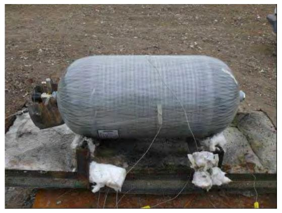
Figure C-1. Overall Setup for Cylinder Bonfire Tests – 5,000-psig Type 3 Cylinder Shown.
