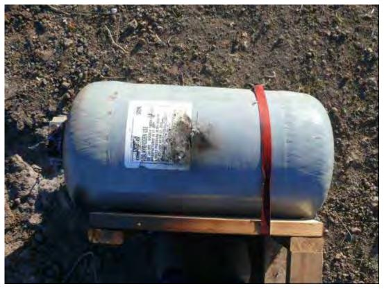
Figure C-13. Hole in 5,000-psig Type 4 Cylinder Following Penetration Test.
