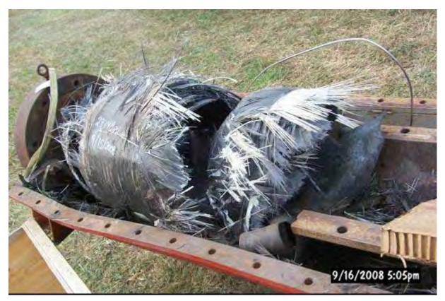
Figure C-10. Typical Failure of Catastrophic Failure Following Burst-Pressure Test.
