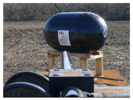
Figure 3. Penetration Test General Setup (Prior to Securing Cylinder to Test Stand).
