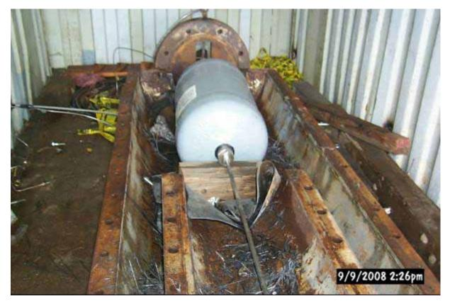
Figure C-9. General Setup for Burst-Pressure Tests. (5,000-psig Type 4 Cylinder Shown)
