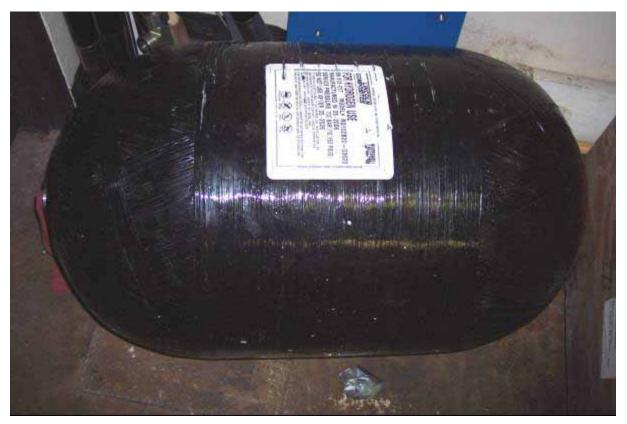
Figure C-7. 10,000-psig Type 4 Cylinder Setup for Pressure Cycling Tests.
