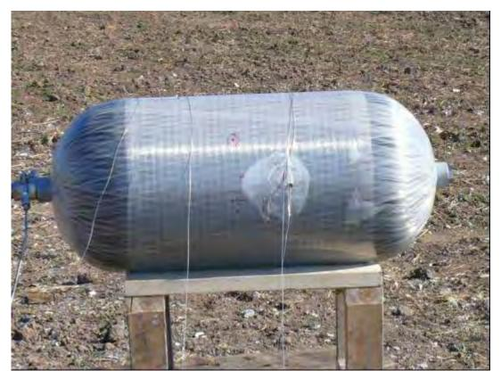
Figure C-12. Hole in 5,000-psig Type 3 Cylinder Following Penetration Test.
