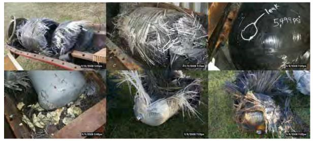
Figure 5. Cylinders Following Burst Pressure Tests. Shown Left to Right, Top to Bottom in Order of Results Table.
