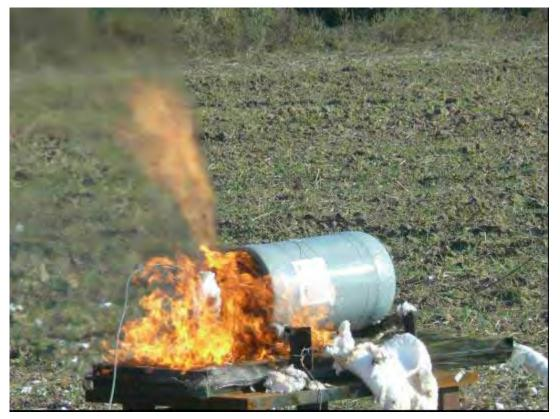
Figure C-3. View of 5,000-psig Type 4 Cylinder Venting.
