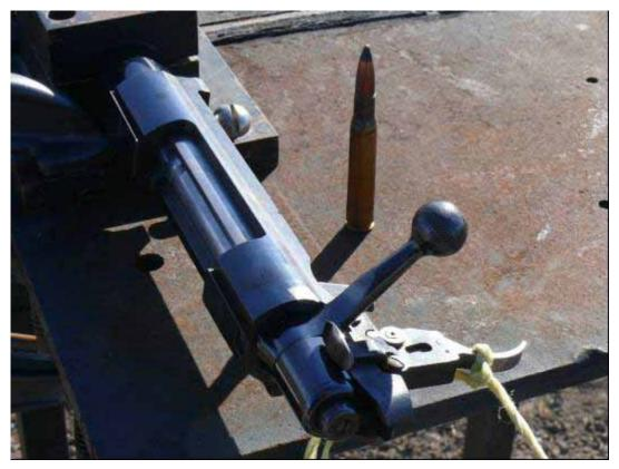
Figure C-11. Gun Bolt and Bullet for Penetration Tests.
