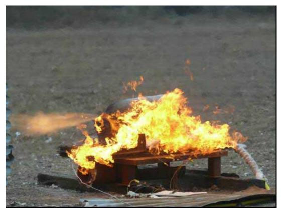
Figure C-2. View of 5,000-psig Type 3 Cylinder Venting.
