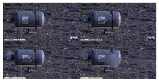
Figure 7. High-Speed Video Frames of 5,000-psig Type 4 Cylinder Penetration Test.
