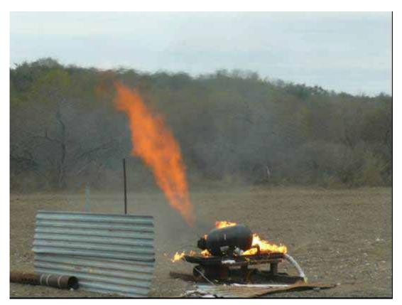
Figure C-4. View of 5,000-psig Type 4 Cylinder Venting.
