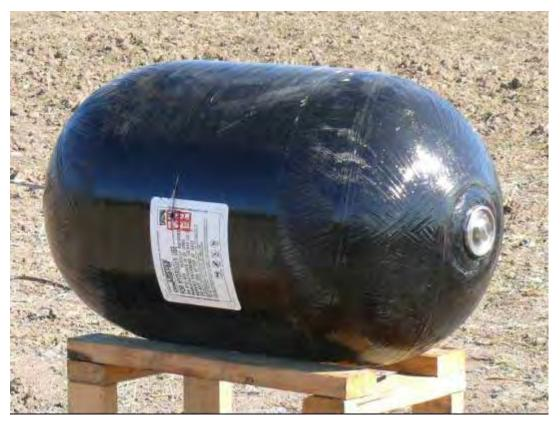
Figure C-14. Hole in 10,000-psig Type 4 Cylinder Following Penetration Test.
