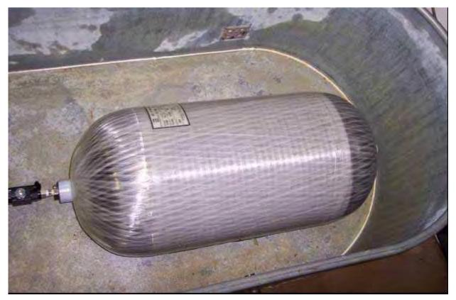
Figure C-5. View of 10,000-psig Type 4 Cylinder Venting.
