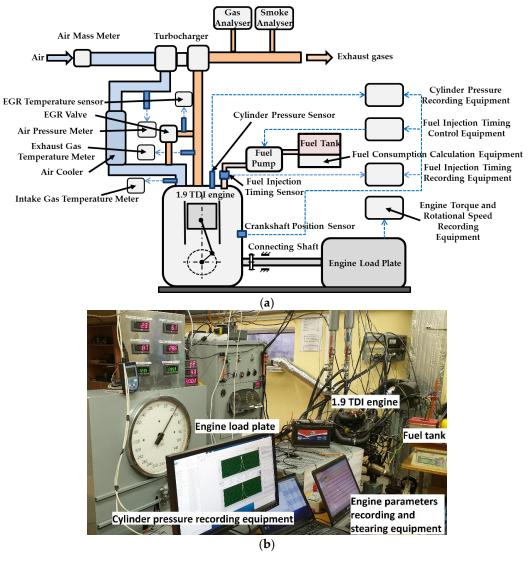
Figure 1. Image of the test engine: (a) test bench scheme; (b) test rig.
