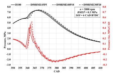
Figure 6. Dependence of pressure and pressure rise in the cylinder on the crank angle degree.
