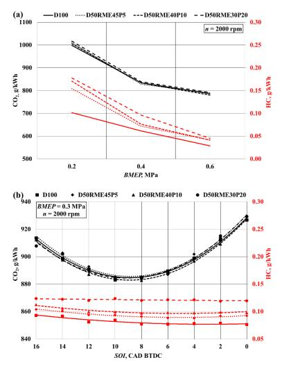
**Figure 4.** Dependence of carbon dioxide emissions and hydrocarbons on different: (a) loads; (b) injection timing.
