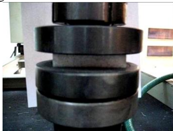
Fig. 2 Compress test fixture of X-Cor sandwich
