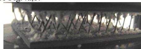
Fig.4a Test result of X-Cor sandwich without foam
