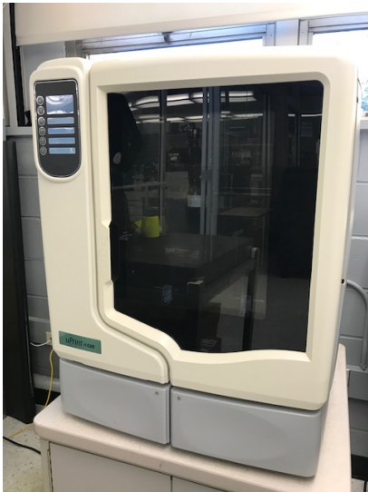
Figure 3. Stratasys uPrint SE Plus Printer
