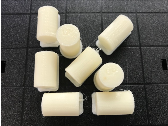
Figure 4. Orientations of Specimens at 3D Printing
