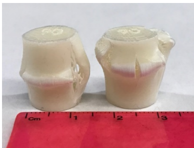
Figure 20. ABS Specimens of Sparse Structure Printed by Mojo at flat-90° Print Orientation After Compression Test.
