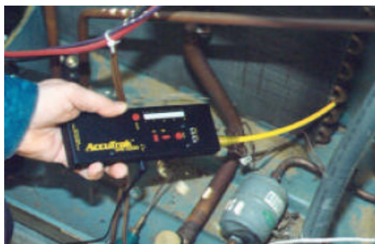
Figure 9. Ultrasonic leak detector (Tashian, Paul)
