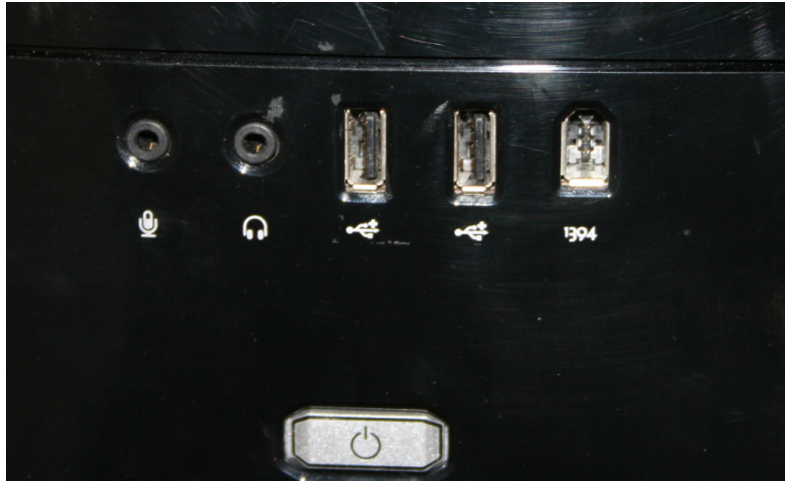
Exhibit: Front panel connectors
