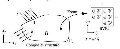
Figure 1: Macroscopic and microscopic structures
