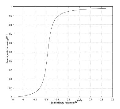
Figure 10: Damage Evolution Law for the Blackglas  $^{TM}$  Matrix
