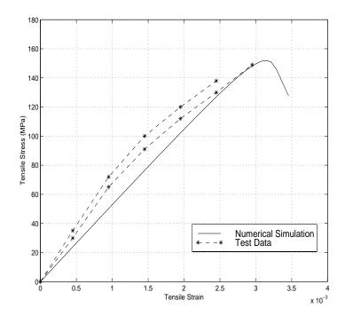
Figure 11: Strain-Stress Curves for the Uniaxial Tension Problem
