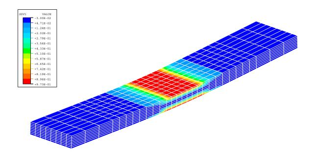
Figure 13: Damage Distribution at the Peak Load in the 4-Point Bending Problem
