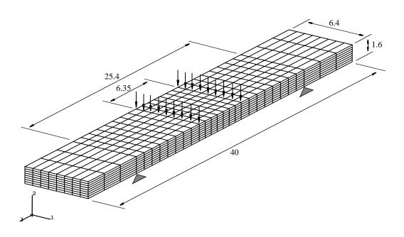
Figure 9: Configuration and FE Mesh of 4-Point Bending Problem
