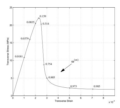
Figure 6: Loading Capacity in the Transverse (X axis) Direction
