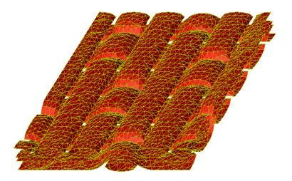
Figure 8: Microstructure of AF10 Woven Composites
