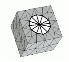
Figure 3: Finite Element Mesh of the RVE for Fibrous Microstructure
