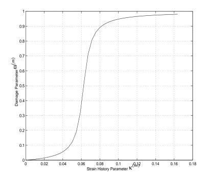
Figure 4: Damage Evolution Law for the Titanium Matrix
