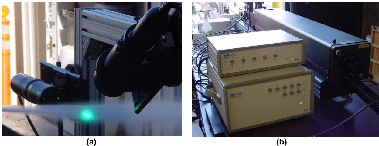
Figure 9. (a) The 2-D PDPA System Measuring the UHP Rosenbauer Water Spray (b) The 2-D PDPA Laser and Multi-channel Signal Processor
