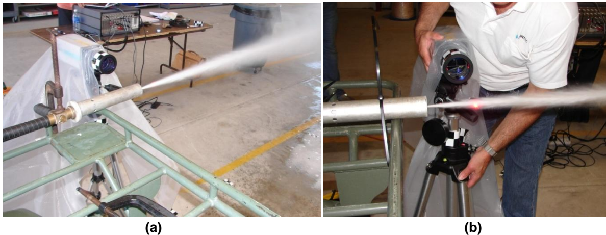
Figure 8. (a) The 6% AFFF UHP FRE Nozzle Accompanied by the 1-D LDV System (b) UHP FRE 1-D LDV System in Action Recording Instantaneous Velocities for the Water Only UHP FRE Spray
