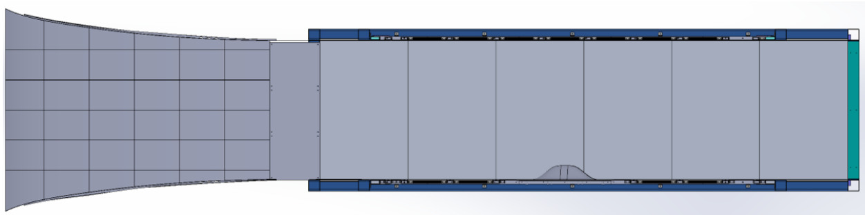
Figure 2.1: The as-designed geometry of the contraction and test section.
