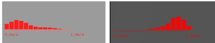
Figure 6. Probability Density Distribution of Wind speed. Left: Existing bus stop design commonly encountered in Singapore. Right: Proposed bus stop design.
