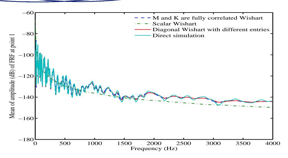
Mean of the amplitude of the response of the cross-FRF of the plate, n=1200,  $\sigma_M=0.078$  and  $\sigma_K=0.205$ .
