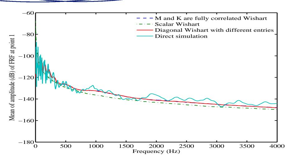
Mean of the amplitude of the response of the cross-FRF of the plate, n=1200,  $\sigma_M=0.133$  and  $\sigma_K=0.420$ .
