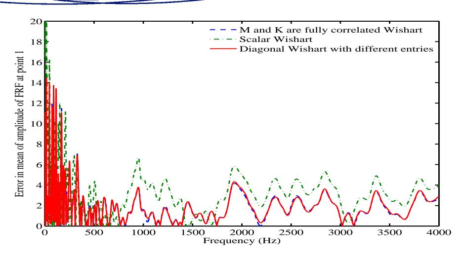
Error in the mean of the amplitude of the response of the cross-FRF of the plate,  $n=1200,\,\sigma_M=0.133$  and  $\sigma_K=0.420.$
