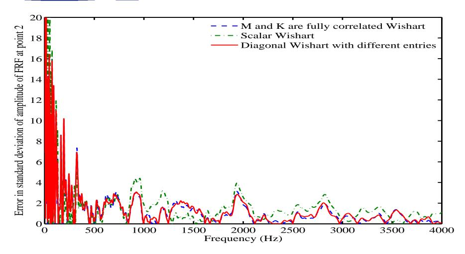
Error in the standard deviation of the amplitude of the response of the driving-point-FRF of the plate,  $n=1200,\,\sigma_M=0.133$  and  $\sigma_K=0.420.$
