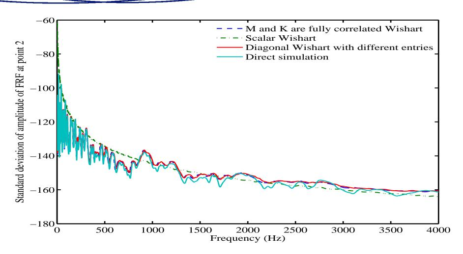
Standard deviation of the amplitude of the response of the driving-point-FRF of the plate,  $n=1200,\,\sigma_M=0.078$  and  $\sigma_K=0.205.$
