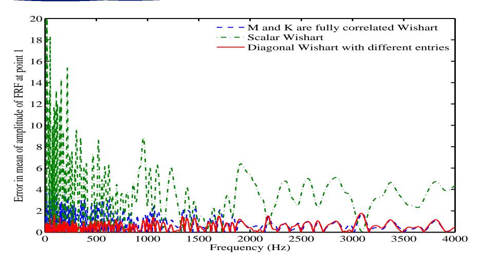
Error in the mean of the amplitude of the response of the cross-FRF of the plate,  $n=1200,\,\sigma_M=0.078$  and  $\sigma_K=0.205.$
