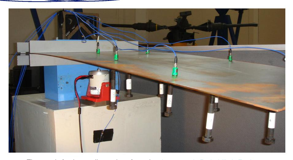
The test rig for the cantilever plate; front view (to appear in Probabilistic Engineering Mechanics).
