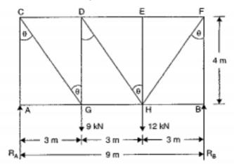
f. A truss is as shown in figure. Find the forces in all members of the truss and indicate it is in tension or compression.
