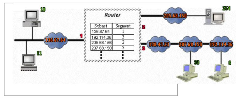
• Routers connect two or more networks and forward data packets between them. When data arrives from one of the segments, the router decides, according to it's routing table, to which segment to forward that data.
