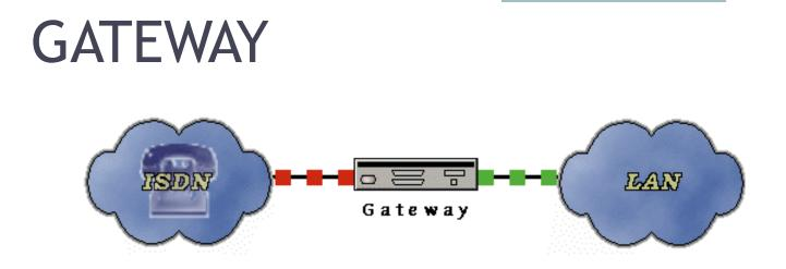
• "Gateway" is a term that was once used to refer to a routing device. Today, in the TCP/IP world, the term "router" is used to describe such a device.
