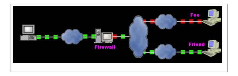
• Firewalls are systems that establish access control policies among networks. They can block information from entering a network or from getting out of that network, they can permit different users to perform different kinds of operations, according to the user's authorizations.
