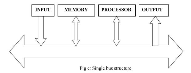
Since the bus can be used for only one transfer at a time, only two units can actively use the bus at any given time. Bus control lines are used to arbitrate multiple requests for use of one bus.
