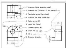
middle and not by interrupting the dimension lines. Here the dimensions can be read from the bottom or from the right side of the drawing.
