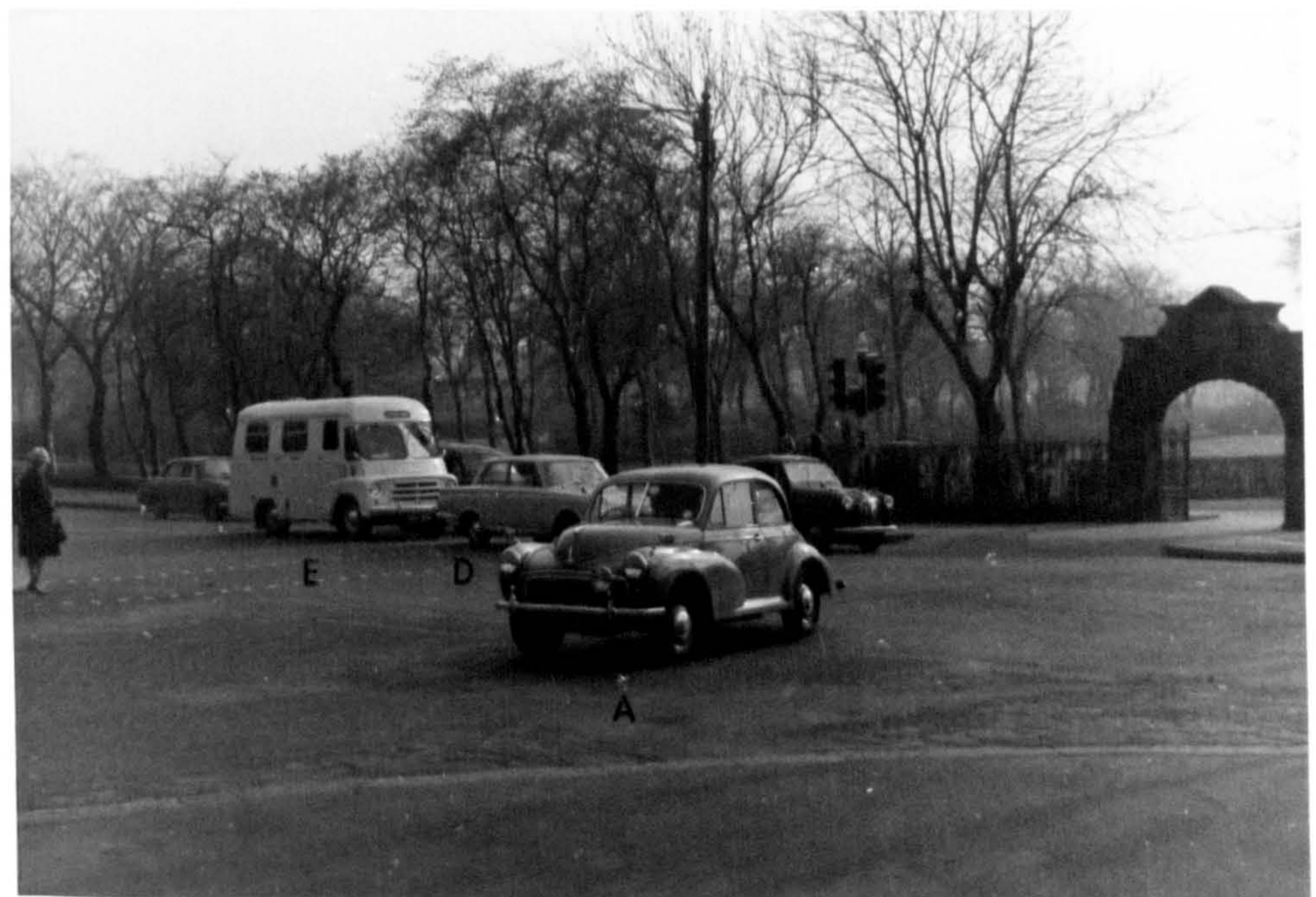
fig. 2.8 Gap measurement using time lapse cinematography
