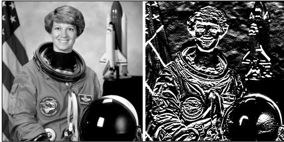
Figure 14: The image on the left is the input image and the image on the right is the output of Sobel in the y direction
