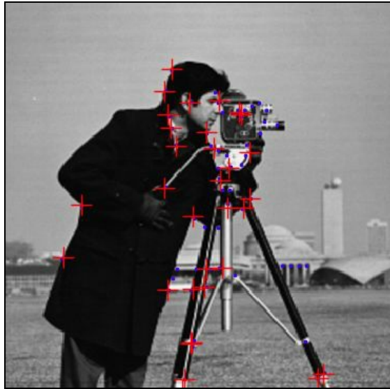
Figure 2: The red cross signs show the corners detected by the Harris corner detector
