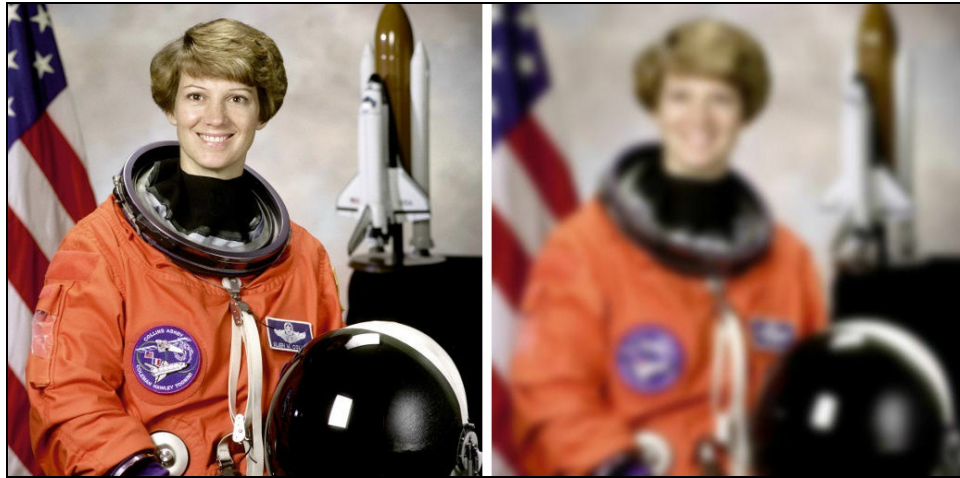
Figure 7: Output of the Gaussian blur using Pillow; the image on the left is the original image and the image on the right is the result of the Gaussian blur
