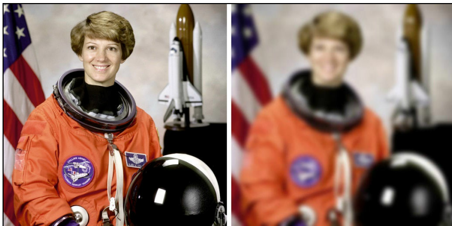
Figure 6: Output of the Gaussian blur using Pillow; the image on the left is the original image and the image on the right is the result of the Gaussian blur
