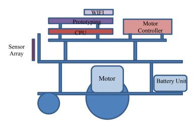
Fig. 2. Schematic diagram of the baseline robot
