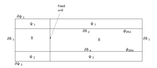
Figure 3: 2D electromechanical actuator model with all the boundaries and domains:  $\delta$  is the polymer domain,  $\psi_1 \& \psi_2$  are the electrode domain,  $\partial \delta_{1-4}$  are the polymer boundaries,  $\phi_{\partial \delta 2} \& \phi_{\partial \delta 4}$  are boundary condition at the electrode-polymer interface,  $\partial \psi_1$  and  $\partial \psi_2$  are boundaries of applied electric potential.
