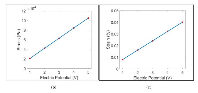
Figure 9: Mechanical response at different electric potential for Nafion actuator:(a)Displacement versus Electric potential (b) Stress versus Electric potential (c) Strain % versus Electric Potential
