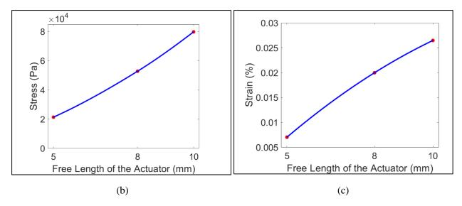
Figure 17: Mechanical response at different actuation length for the TMD-Nafion actuator: (a) Actuation length vs Displacement (b) Stress vs Actuation Length (c) Strain % vs Actuation Lengths.
