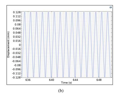
*Figure 6: Tip displacement of the Nafion actuator under applied potential.(a) Displacement vs Time under 2V 1Hz square signal (b) Zoomed image of the tip displacement*
