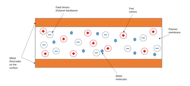
Figure 1: Conceptual diagram of the actuator
