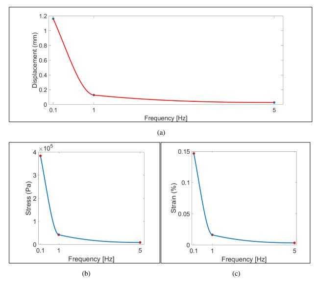
Figure 10: Mechanical response at different excitation frequencies for Nafion actuator:(a)Displacement versus frequency(b) Stress versus frequency (c) Strain % versus frequency
