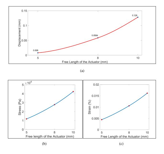
Figure 11: Mechanical response at different actuation length for the Nafion actuator: (a) Actuation length vs Displacement (b) Stress vs Actuation Length (c) Strain % vs Actuation Lengths
