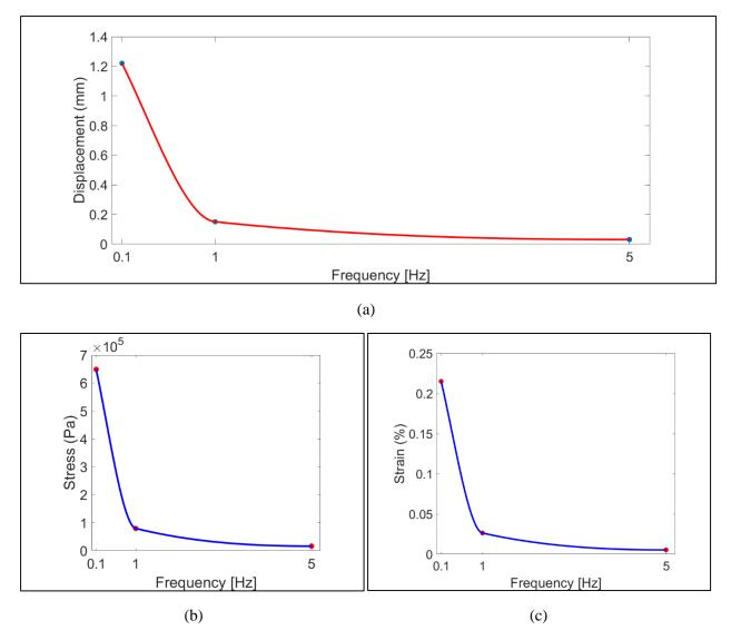
Figure 16: Mechanical response at different excitation frequencies for TMD-Nafion actuator:(a)Displacement versus frequency(b) Stress versus frequency (c) Strain % versus frequency
