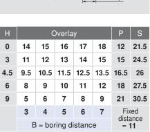
NOTE: 4.5 plate is only for use in frame cabinets, 9 plate is only for panel cabinets
