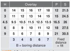
NOTE: 4.5 plate is only for use in frame cabinets, 9 plate is only for panel cabinets
