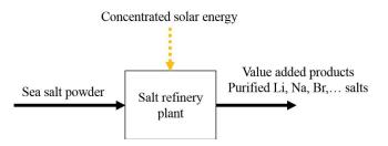
Fig. 6. Production of value-added product downstream of a water desalination plant.
