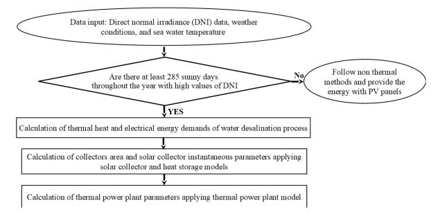
Fig. 1. Methodology of energy and process assessment for water desalination based on CSTC.
