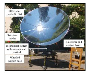
Fig. 7. An off-center parabolic dish concentrator for solar high-temperature studies.
