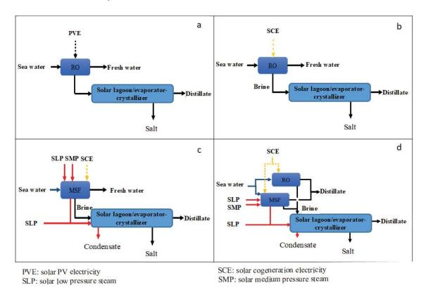
Fig. 2. Different scenarios of water desalination applying solar energy.
