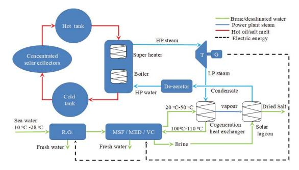
Fig. 3. CSTC desalination plant with heat storage.
