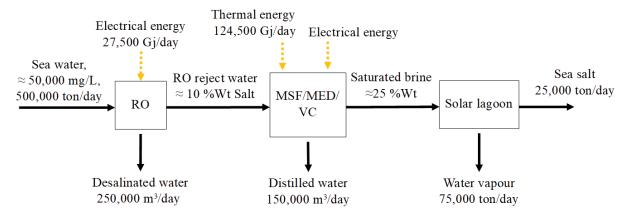
Fig. 5. Mass and energy balance results of ZLD solar desalination plant, winter.
