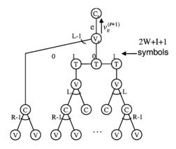
**Figure 2.3:** Message flow neighborhood of depth 1. This figure corresponds to the parameters  $(I, W, d_v = L, d_c = R) = (1, 1, 2, 3)$ .
