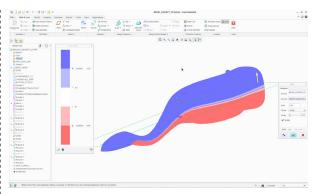
At any point in the process, Creo's set of mould design tools can be used to perform draft and thickness analysis to ensure that the end result is not only aesthetically pleasing, but can be manufactured Ð
