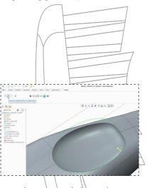
Here the power switch area has been recessed by removing the sub division surface primitive from the model, giving a smooth area
