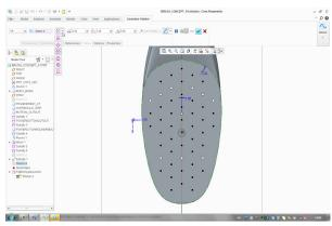
Fill Patterns provide a wide range of possible patterns for bristle positioning. These can be driven by a standard form (such a linear, circular, spiral or angular) or using tabular information for positioning
