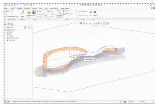
Creo's Trace Sketch tools can arrange drawings to provide a reference for the Freestyle modelling tools. Each plane can be adjusted to the correct size
