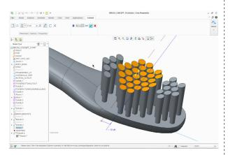
Fill Patterns can also be used to drive feature or part placement as shown with the bristle features. More regular features such as protrusions, cuts and revolves can then be used to add additional form where required
