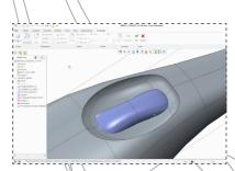
6 A second Freestyle feature is used to create a rocker switch cover intended for over moulding in a more flexible material
