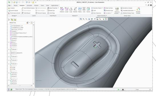
The recessed rocker switch cover and product details (on/off switch) are all added into the model with minimum feature overhead. The recess has been created in a single feature. With traditional modelling methods (either surface or solidbased) this would have been problematic to create and not offer as much in terms of editability. Three additional features and this portion of the concept is complete
