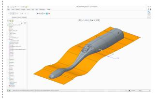
The benefit of using integrated tools for concept design is that the surfaces can be taken through into the detailed design and engineering development. Here the split line is found in the direction of draw and a parting surface is built to assist with tooling design
