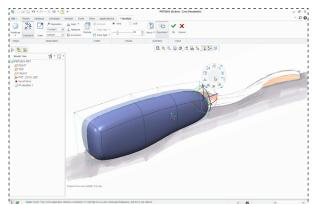
Surfaces are edited using drag and drop of edges, faces and vertices of the control cage. The influence of each entity can be adjusted to build in hard edges
