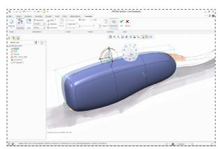
2 Freestyle allows the use of a primitive as the base feature. Automatic mirroring means that symmetry can be maintained in the model where needed, saving lengthy set-ups to control tangency and curvature continuity
