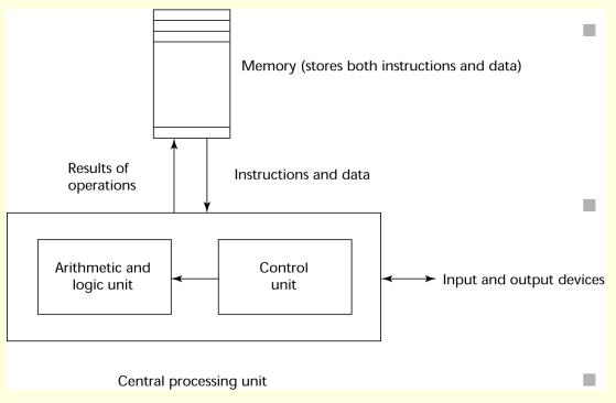
Connection speed between a computer's memory and its processor determines the speed of a computer
