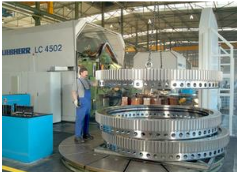
Figure 8. Piling of three roller bearings recently manufactured by Liebherr, Germany[6].
