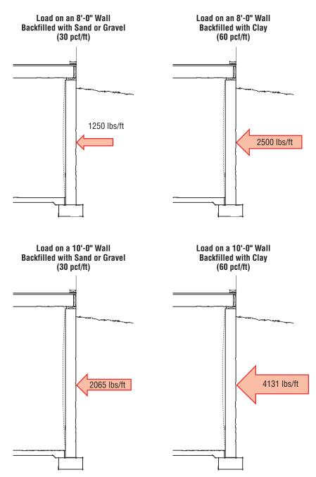
**Figure 2.** Soil type and backfill height both affect the lateral pressure on a basement wall. Backfilling with a clay soil instead of sand can increase the load by double or more, while going from an 8-foot to a 10-foot wall, just a 25% height increase, adds 50% to the lateral pressure. Taller walls backfilled with heavier soil risk failure unless correct design methods are followed.
