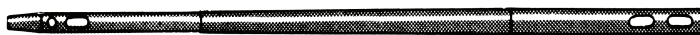
One-piece taper tie with slotted ends to be withdrawn for repeated use. Additional slot for two wall sizes.
