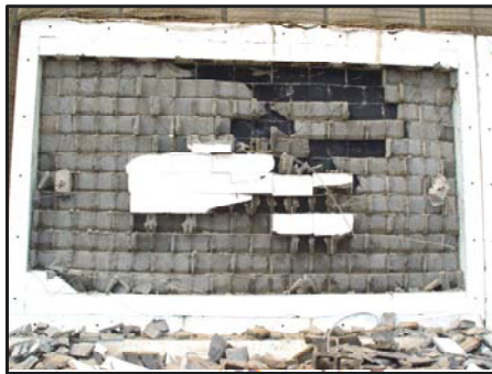
Fig 13. Post-test view of R9, the trowel-on polyurea.
