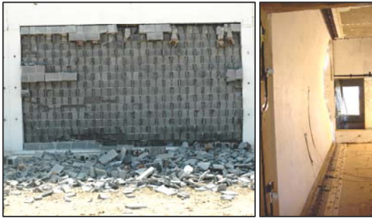
Fig. 12. Post-test view of R8, the spray-on polyurea wall.
