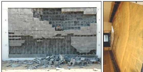
Fig. 14. Post-test view of R10, the trowel-on polyurea and film material.
