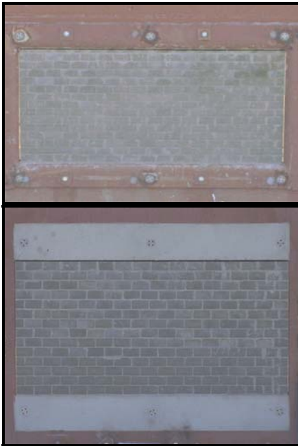
Fig. 1. 1/4-scale CMU wall steel and concrete frame.
