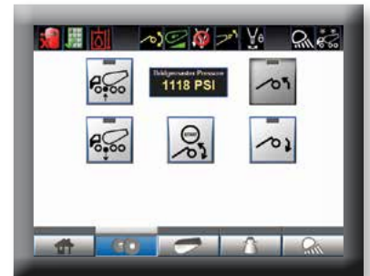
Lift axle controls with Bridgemaster pressure monitoring (option)
