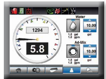
Available digital slump readout and water/chemical add controls
