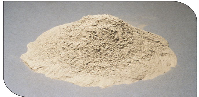
Figure 1. Fly ash, a powder resembling cement, has been used in concrete since the 1930s. (IMG12190)
