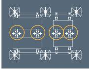
Linear Adjustment The cross bars supporting the equipment unit can slide along the end bars into position required, then be locked in place.
