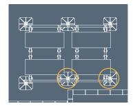
Leg Assembly Positioning The leg assembly is typically positioned outside the frame work, but can be placed inside the framework to avoid an obstruction.
