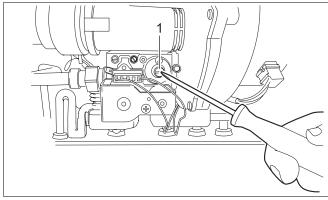
Fig. 37 Setting the gas/air ratio
