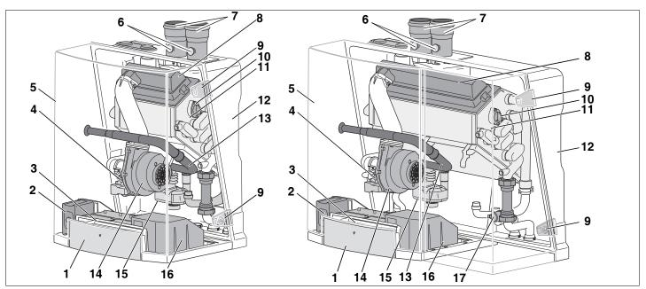
Fig. 1 Logamax plus GB142-24/30 (left) and GB142-45/60 (right)
