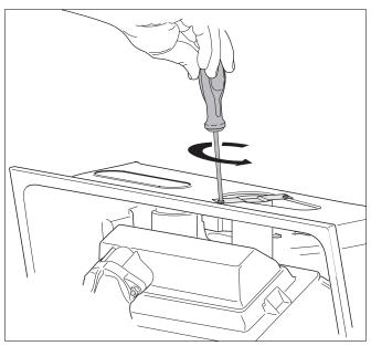
Fig. 13 Removing the transport safety device
