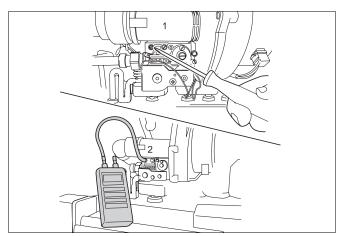
Fig. 34 Measuring the inlet gas pressure
