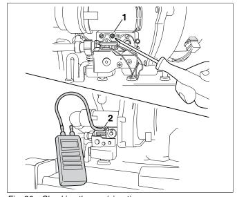
Fig. 36 Checking the gas/air ratio
