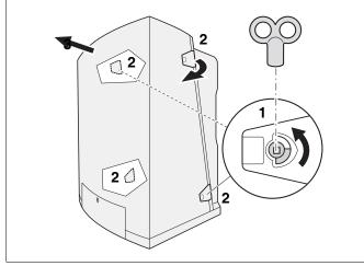
Fig. 7 Removing the casing
