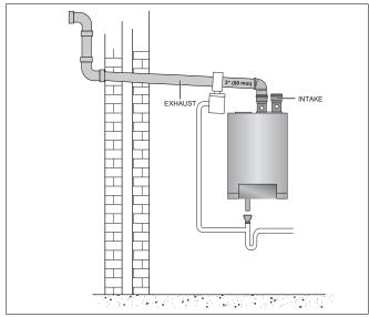
Fig. 27 Condensate drain
