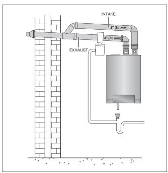
Fig. 26 Horizontal venting system (sealed combustion)
