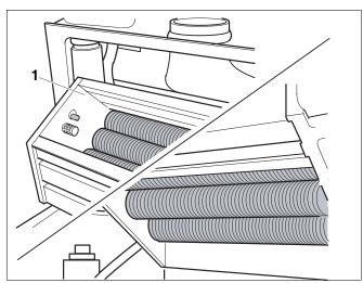
Fig. 47 Cleaning the heat exchanger
