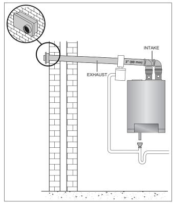
Fig. 21 Horizontal venting system (sealed combustion) - Situation 2
