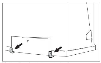
Fig. 6 Removing the transport safety clamps
