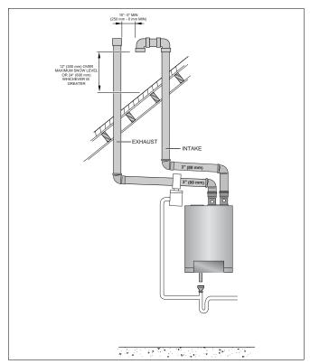
Fig. 22 Vertical parallel venting system (sealed combustion) - Situation 2
