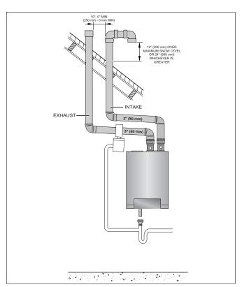
Fig. 20 Vertical parallel venting system (sealed combustion) - Situation 1
