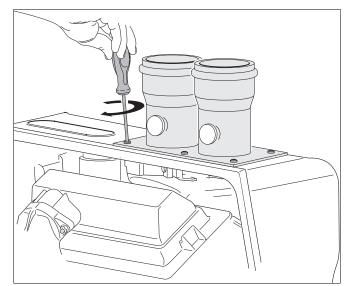
Fig. 14 Connecting the flue gas adapter
