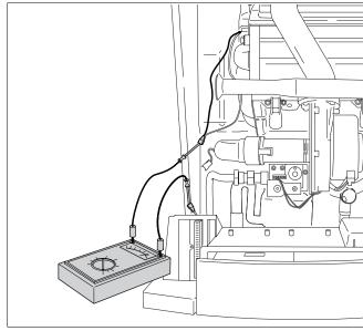
Fig. 39 Measuring the ionization current
