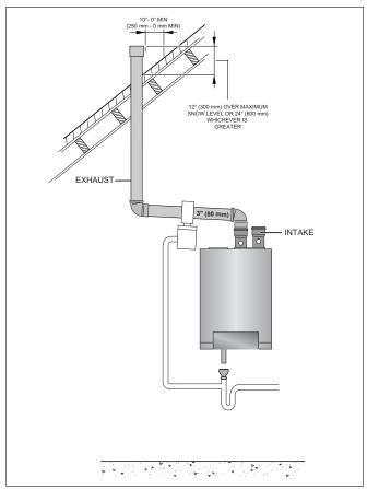
Fig. 24 Vertical venting system (room air only)
