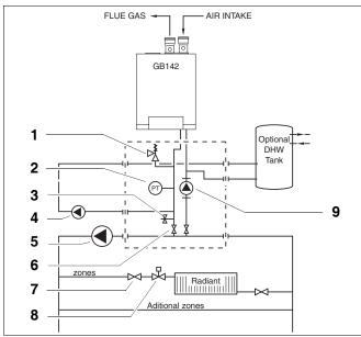
Schematic representation of the boiler with the Fig. 11 hydraulic set connected to an optional hot water tank with one or multiple zones including one pump and zone valves
