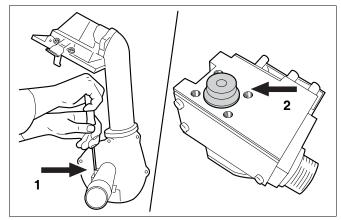
Fig. 50 Replacing the gas orifice
