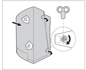
Fig. 41 Installing the casing
