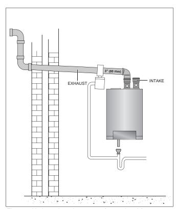
Fig. 19 Horizontal venting system (room air only) - Situation 1
