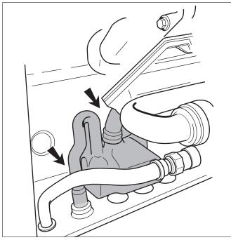
Fig. 32 Filling water into the condensate trap
