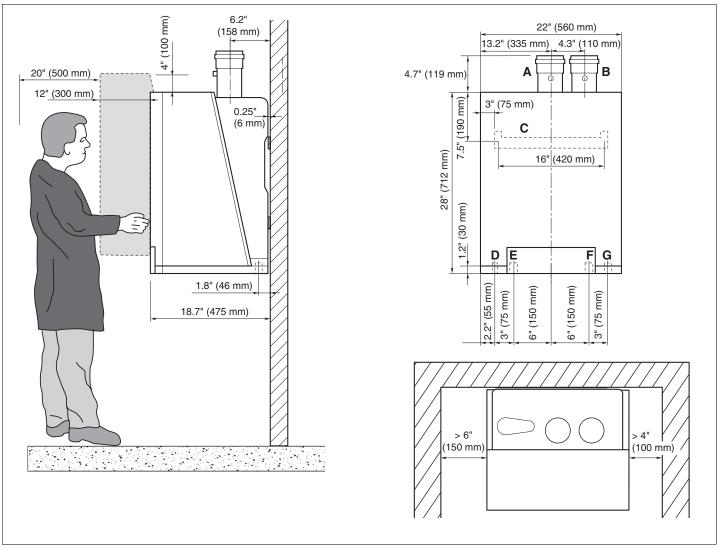
Fig. 3 Dimensions and connections for boiler GB142-24/30 (dimensions in inches)
