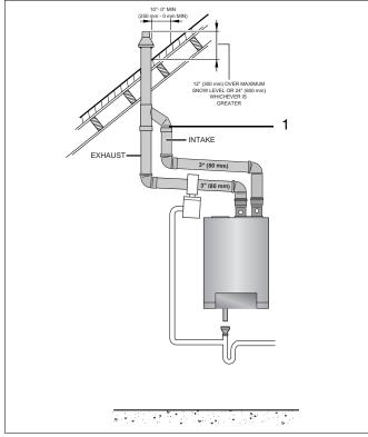
Fig. 18 Vertical venting system (sealed combustion)
