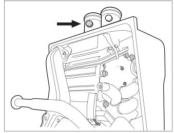
Fig. 38 Flue gas sampling point
