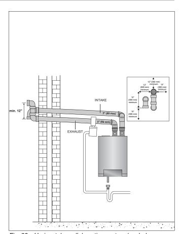
Fig. 23 Horizontal parallel venting system (sealed combustion)
