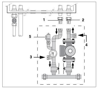
Fig. 9 Pump manifold installation
