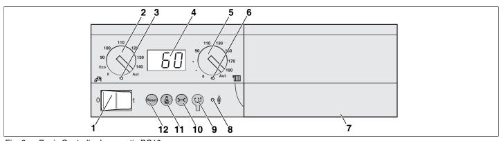
Fig. 2 Basic Controller Logamatic BC10
