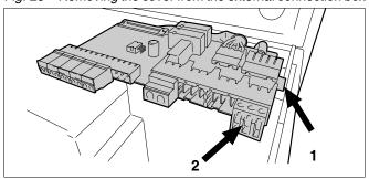
Fig. 29 external connection board
