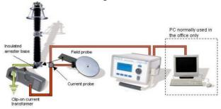
switch yard conditions without any need for shut down. The system is based on the measurement of 3<sup>rd</sup> harmonic resistive current with compensation for harmonic in the system voltage.
