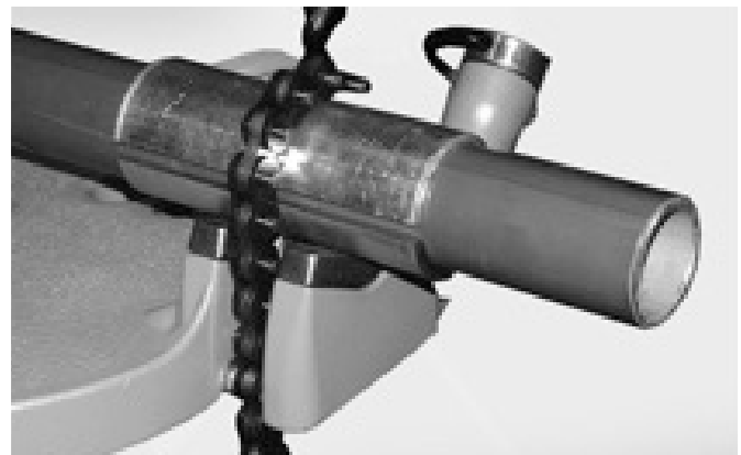
Figure 15: Field-fabricated half shell clamps used with chain vise to protect PVC-Coated conduit.
