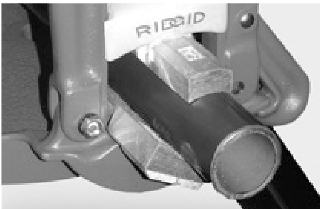
Figure 14: Commercial yoke vise used to protect the PVC coating of PVC-coated conduit.
