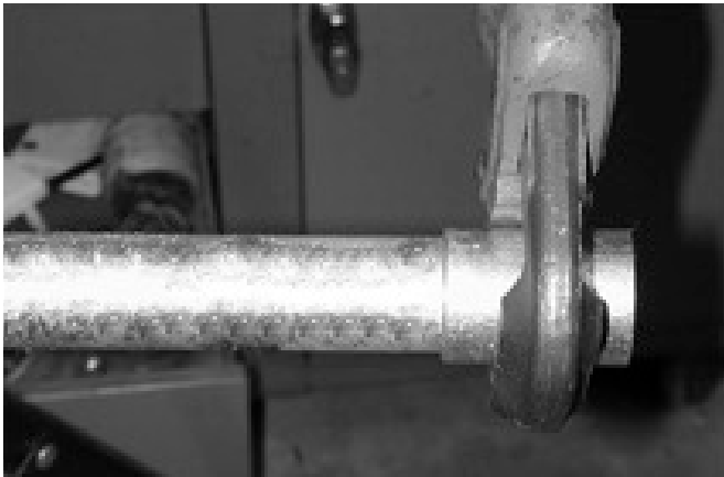
Figure 13: The coupling must be assembled wrench tight.
