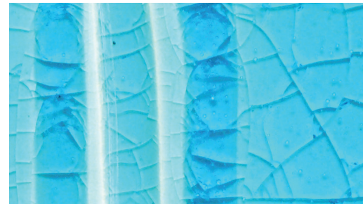
Water Blue with 5% Zircopax and 5% silica added. Results: Largest pattern of crazing.
