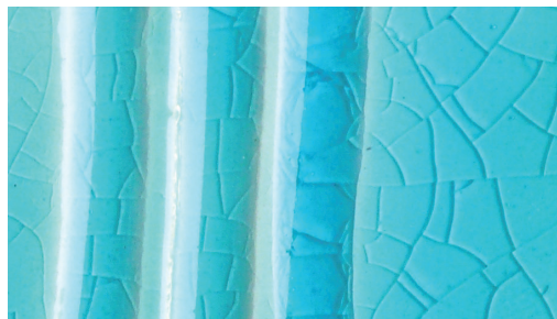
Water Blue with 5% silica added and 5% less Ferro frit 3110. Results: Larger, more spaced out crazing.
