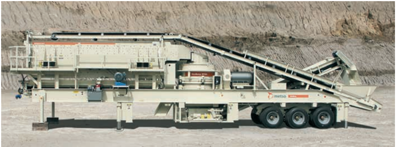
Mobile : The NW300HP is a highly mobile, closed-circuit crushing and screening plant. Ideal for contractors, it can transform your feed stock into three finished fractions.
