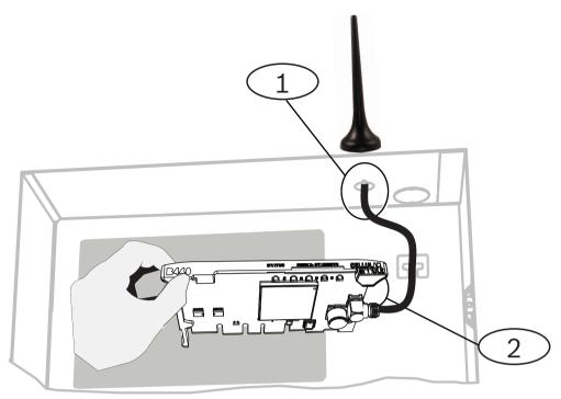
Figure 3.2: Installing the antenna
