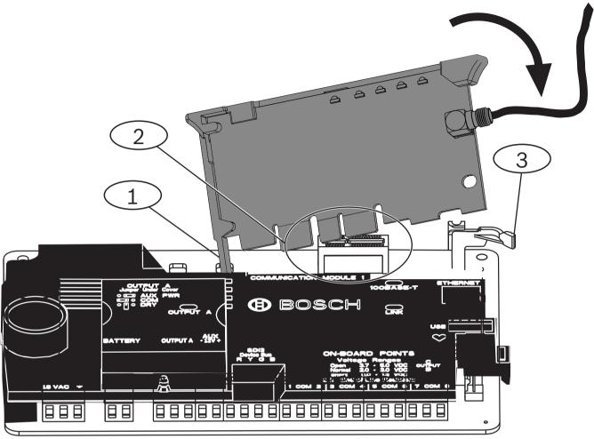
Figure 3.5: Communicator installation (B6512 control panel shown)
