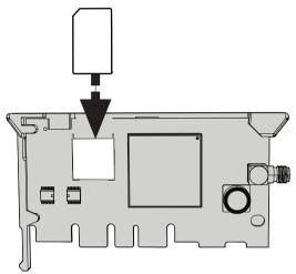
Figure 3.1: Inserting the SIM card
