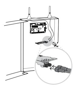
Figure 3.4: B444-A/B444-V cable connection
