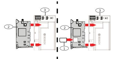
Figure 3.6: Communicator installation (B450 shown)
