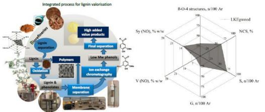
Figure 1. Integrated process for lignin valorization
