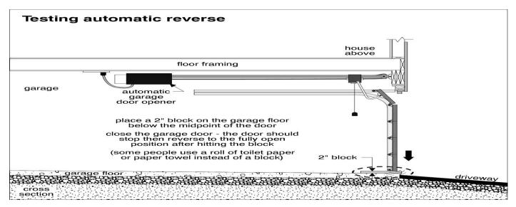
BOTH GARAGE DOOR OPENER SAFETY STOPS SHOULD BE ADJUSTED OR REPAIRED AS IS FOUND TO BE REQUIRED TO ENSURE A PROPER SETTING OF APPROXIMATELY TEN POUNDS OF RESISTANCE PRESSURE TO RETURN THE DOOR TO AN OPEN POSITION.
